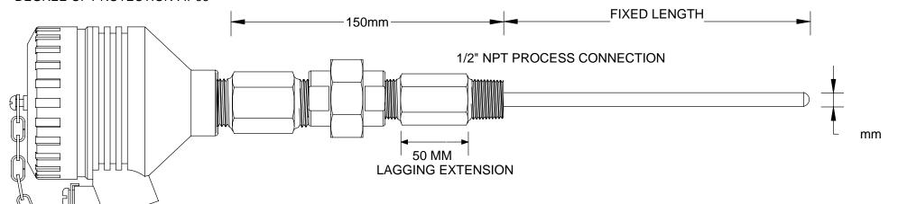
CERTIFIED FOR USE WITH MIMS THERMOCOUPLES AND MIMS RTD SENSORS
